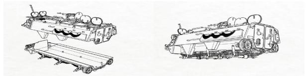
Wheel assembly as layers, note that last axle is not steerable and it has different inside. Sprue C
