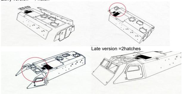
Body parts are on sprue A and D. If you build the earlier version, use roof part with only one hatch above driver's place.
