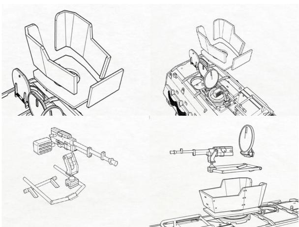
Gun shield is used in some versions, parts are from sprue D. Machine gun from sprue B. Check references for the version you are building if this is used or not. This is used with Danish, Norwegian, Estonian and Swedish vehicles. **Instruction to build ambulance.** Use part from sprue D to close gunners hatch. Large box is for Finnish military and Finnish
