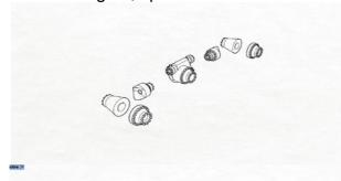
All parts are on sprue E. Cut the axle 3-4mm from right side, add differential and glue axles together, Notice, that you measure length of the axle (see measurements below).
